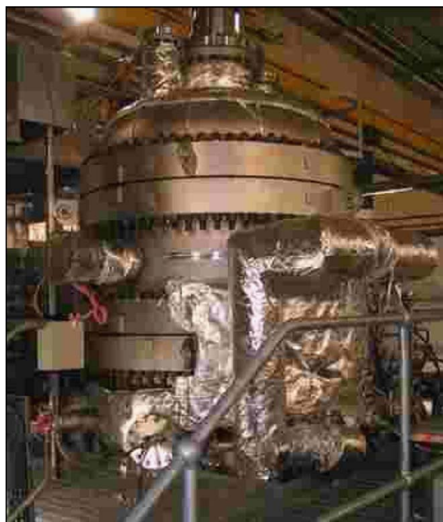
Fig. 5. Pressurised rig for testing 10 kW e stack blocks.
